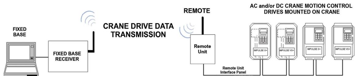
With crane control system data transmission, users do not have to be in close proximity to the crane to detect a possible problem, which means less exposure to the hot metal environment and a shorter response time to resolve an issue.
